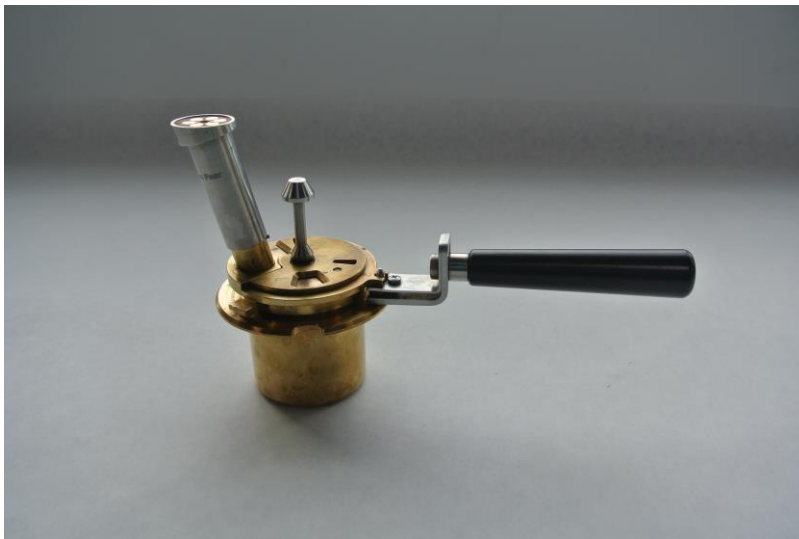
Photograph 7 - Closed cup with electrolyte for flash point testing
