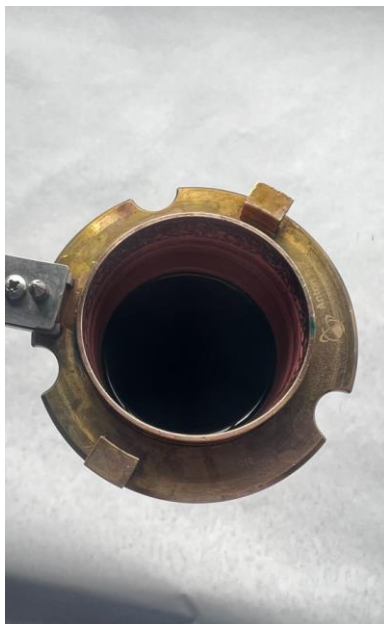
Photograph 11 - Electrolyte in the cup after flash point test
