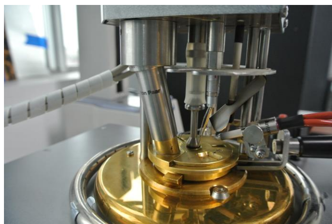
Photograph 10 - Flash point test setup with Igniter
