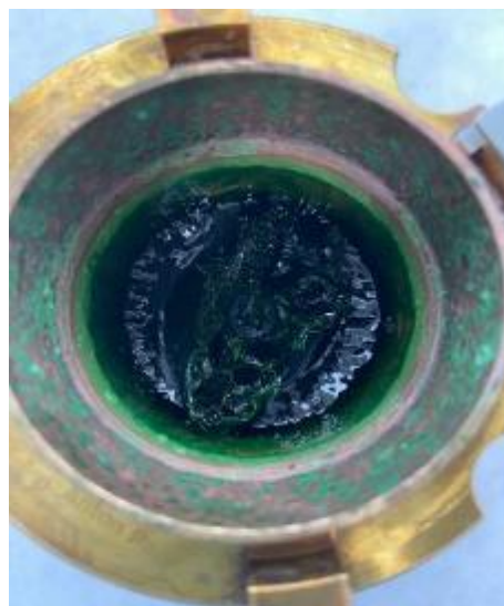
Photograph 6 - Electrolyte in the cup after flash point test - View 2
