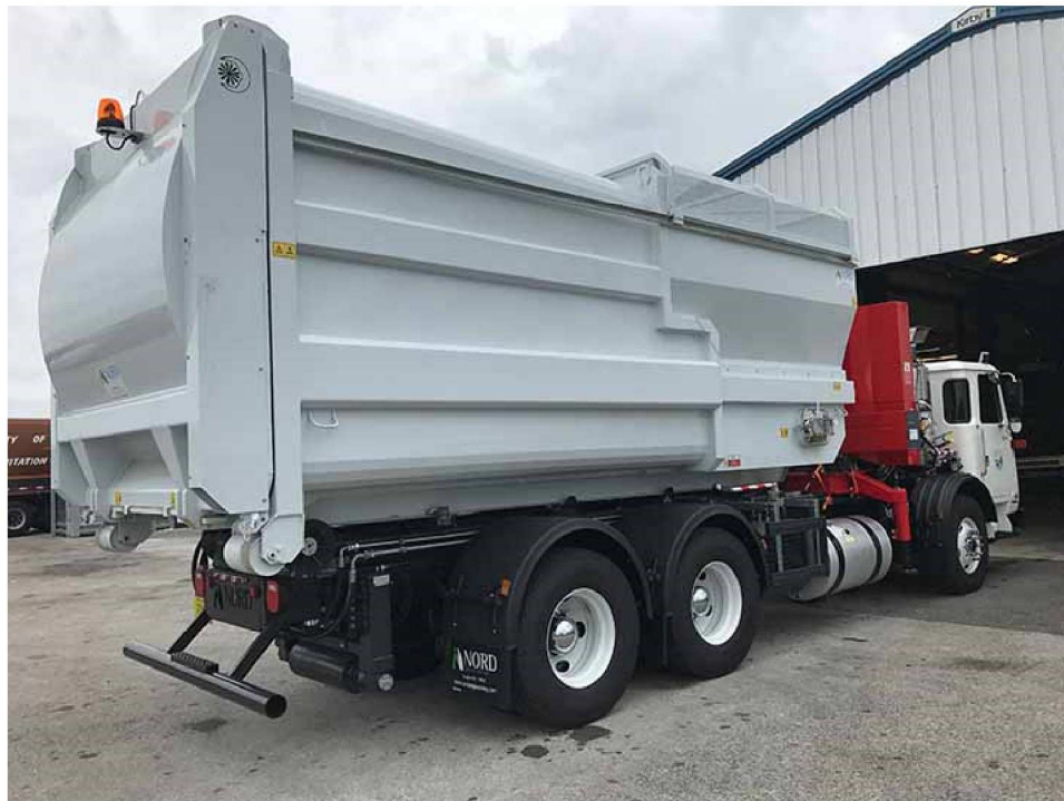
US Truck Chassis with Italian Lift and Compactor used in Florida.
